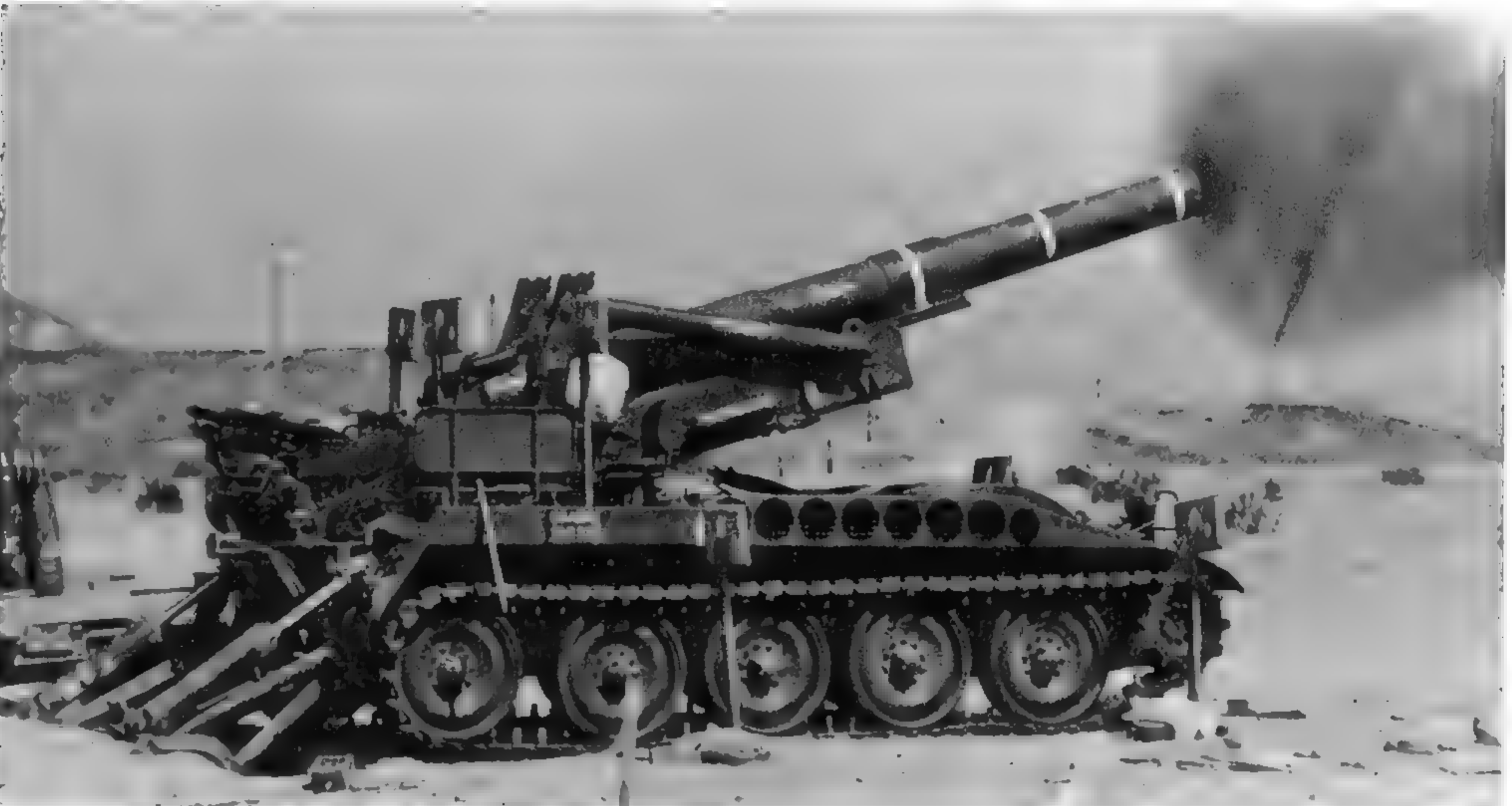
This M110 is firing on the range at Yuma during tests. The radical difference in barrel length between the original configuration of the M110 and the M107 is readily apparent. (U.S. Army photo)
